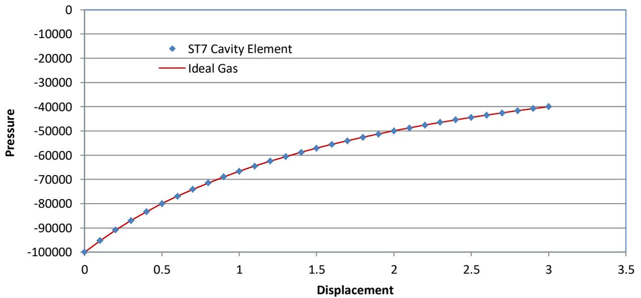
Case 2: Decreasing the volume by enforced displacements and monitoring the cavity pressure.
