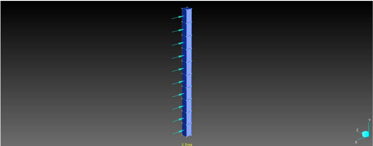
A Factor vs Velocity table controls the aerodynamic drag force.
