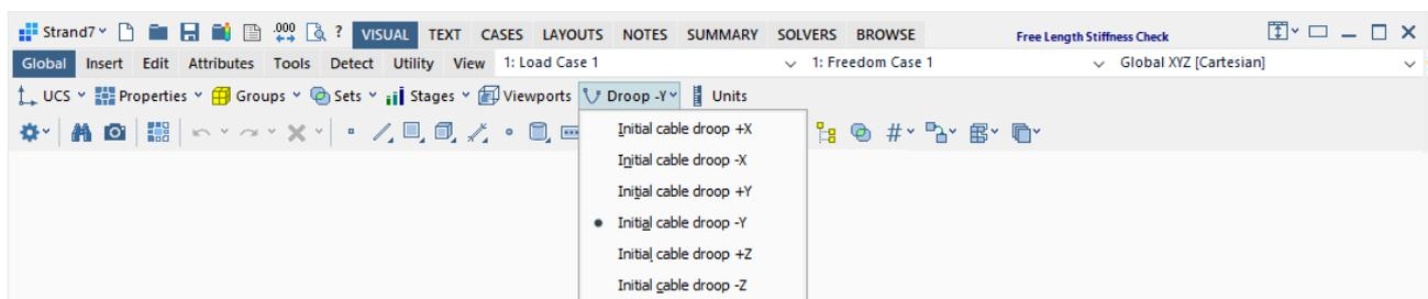
The initial shape is determined by solving the catenary equation for an inextensible cable of the prescribed length, drooped in the nominated direction. This then becomes the zero-displacement position in the analysis. Displacements produced by the various solvers are then assumed to be with reference to this initial shape (i.e., position) and therefore cable displacements, in addition to cable positions, can be determined even for the first load step of an analysis.
