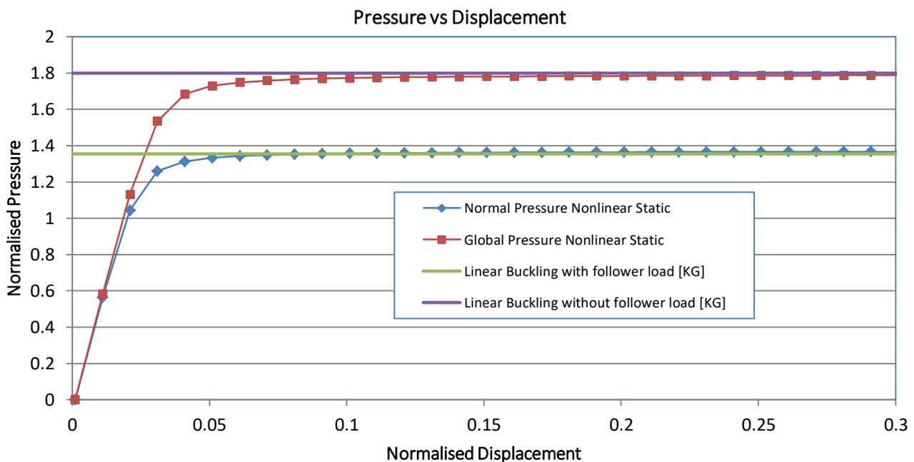
Note that in general, the load stiffness matrix is non-symmetric. However, a symmetric approximation has to be included in linear Eigenvalue solvers that work only with symmetric matrices. The accuracy and applicability of this option should be checked with the GNL solver as in the example above.
