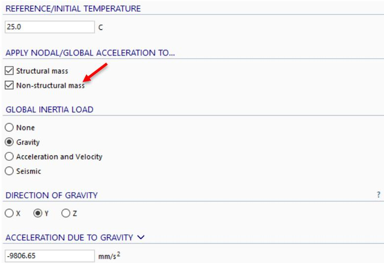
The inclusion of non-structural mass in the global mass matrix is set on the **SOLVERS/Home** tab of the dynamic solvers.
