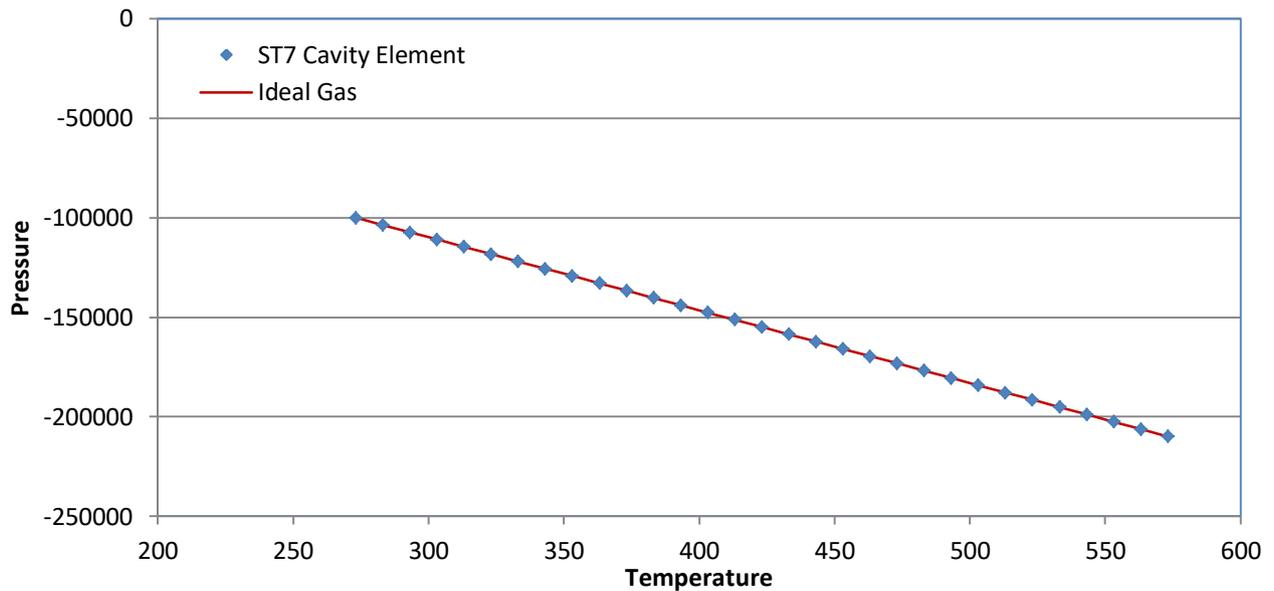
The above graphs report the pressure acting on the plate (or brick) surfaces. For an ideal gas cavity, the element surface pressure will range between zero (i.e., a vacuum) and some negative number (i.e., a compressive pressure on the surface).
