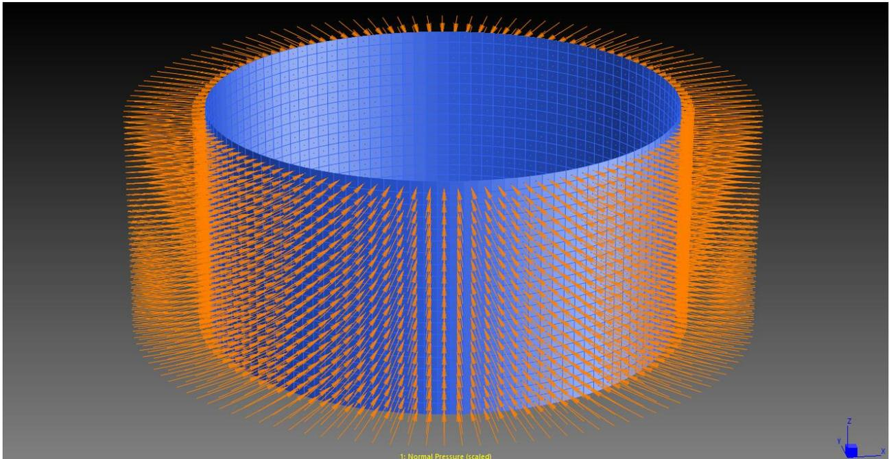
In addition to the nonlinear static analysis, two linear buckling analyses are conducted using the load case with normal pressure attributes: one analysis includes the follower load [KG] whilst the other does not.
