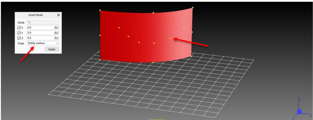
This tool also offers an **Edit** option that allows for an existing node to be moved from its current location onto a grid point, a vertex or another node: click to pick up the source node and click to drop the node onto the other entity.
