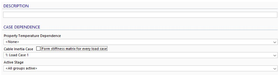
This is required because the stiffness of a cable element depends on its catenary shape, which is determined by the applied inertia loads acting on the mass of the cable, together with the stiffness of the structure to which the cable ends are attached.
