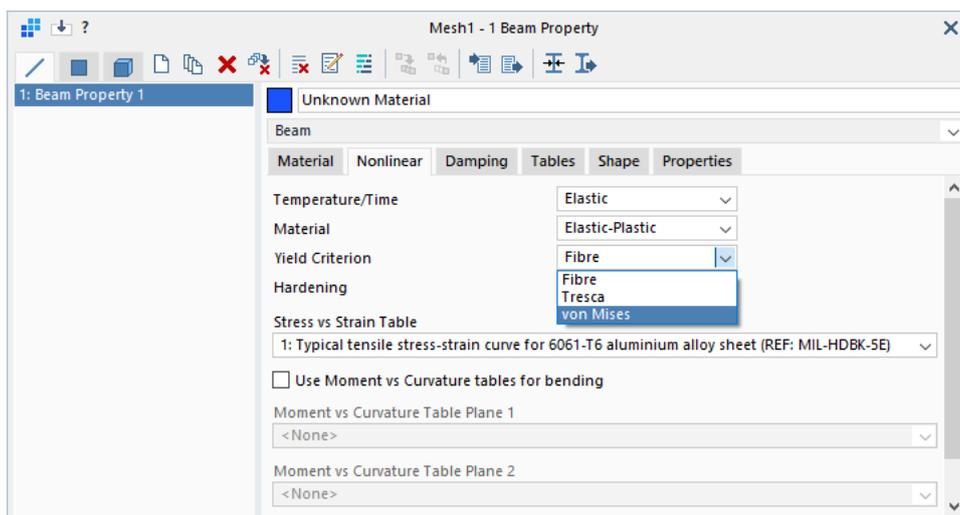
The use of the von Mises criterion in a material nonlinear analysis is demonstrated via the simple example below whereby the results of a single beam element with a rectangular solid cross section under torque, applied as an enforced rotation, are compared with an equivalent brick element model. The material is assumed to be elastic-perfectly-plastic.
