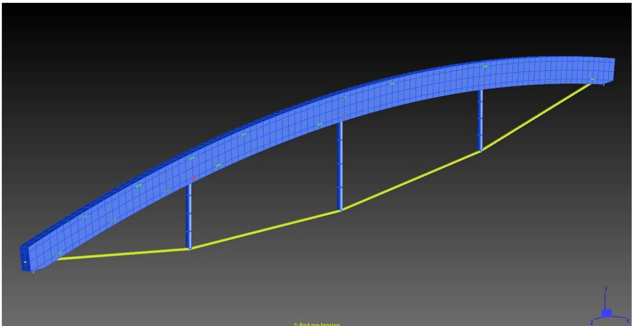
The model is set up with three load cases: gravity, pre-tension and roof load. A linear static analysis calculates the results for these load cases. A combination case is defined to combine gravity and pre-tension into one result case. The linear buckling analysis then selects the combination case as the **Constant Case** and the roof load case as the **Variable Case**. The buckling factors calculated scale the roof load while the other loads are applied unscaled.
