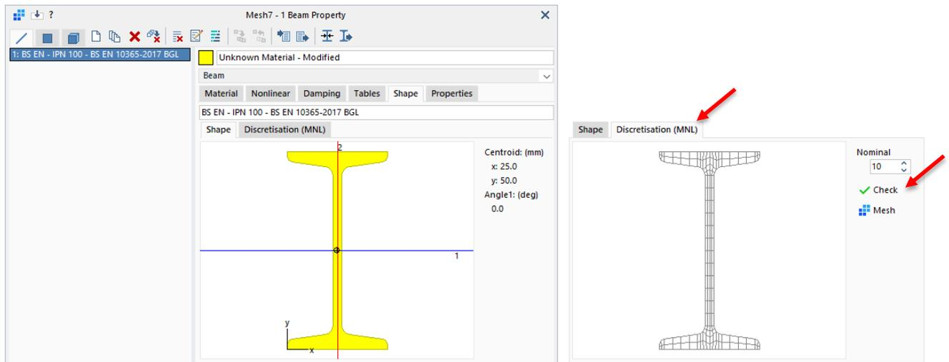
As the coefficients can only be calculated at a pre-defined number of points on the section, a balance needs to be found between accuracy of results and calculation time. This can depend on the section shape and the type of load applied. The **Shape/Discretisation** tab of the beam property dialog provides a tool to **Check** the quality of the mesh and the shear stress integration for different levels of discretisation.
