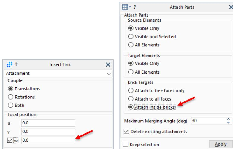
For example, this feature offers the possibility of easily connecting beam elements representing steel reinforcement to the inside of a brick mesh representing concrete, without the need for a compatible mesh between the beam and the brick elements.
