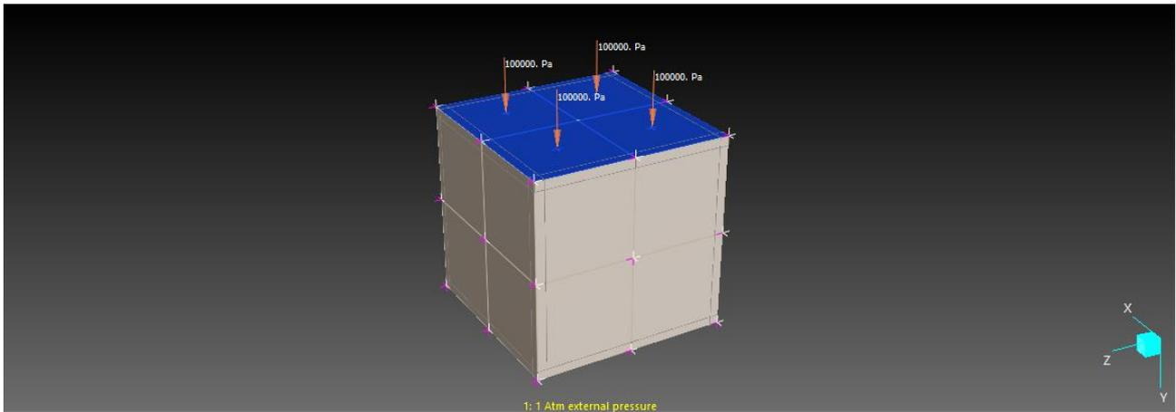
Case 1: Increasing the volume by enforced displacements and monitoring the cavity pressure.
