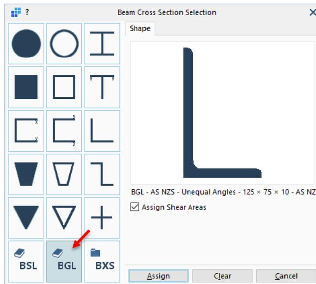
Cross sections in the BGL consider a more detailed geometry than the simplified six-parameter definition of section shapes in the BSL. BGL sections take into account the root and toe radii, flange tapers and more. These allow for a better representation of the geometry for more accurate evaluation of shear stress and nonlinear material behaviour.
