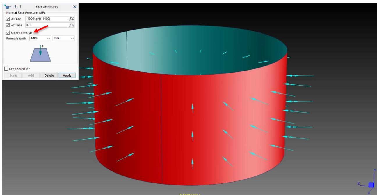
When the faces are meshed, the elements evaluate the formula so that each element has the correct value of pressure assigned.
