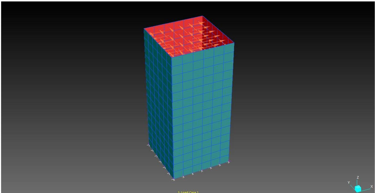
A Factor vs Position table is defined to represent water pressure with depth.
