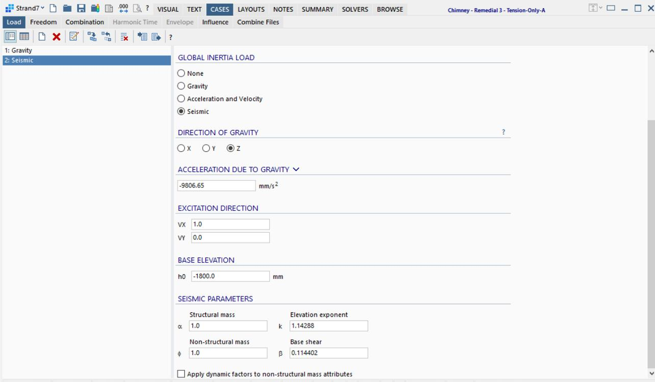
The screenshot shows the Strand7 software interface with the 'CASES' tab active. The 'Seismic' load case is selected. The 'GLOBAL INERTIA LOAD' settings are as follows:
