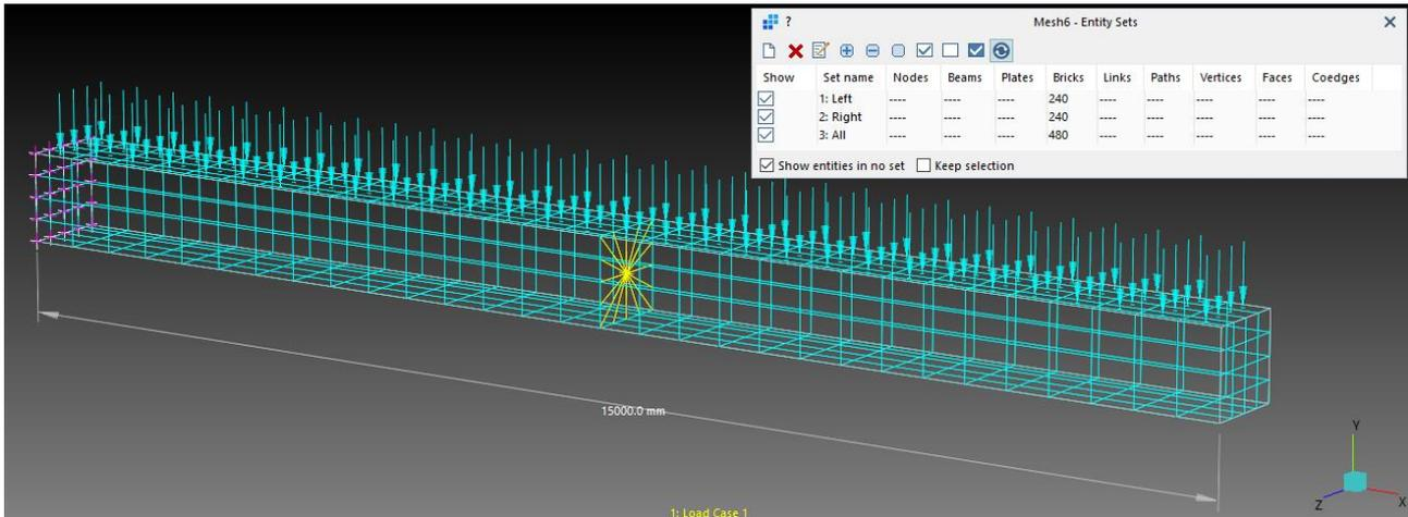
A linear static analysis is executed and the forces and moments at the Reaction MPL are extracted using **Peek**. Three cases are considered; in each case one of the entity sets is assigned to the MPL before extracting the results. The MPL forces are tabulated below.
