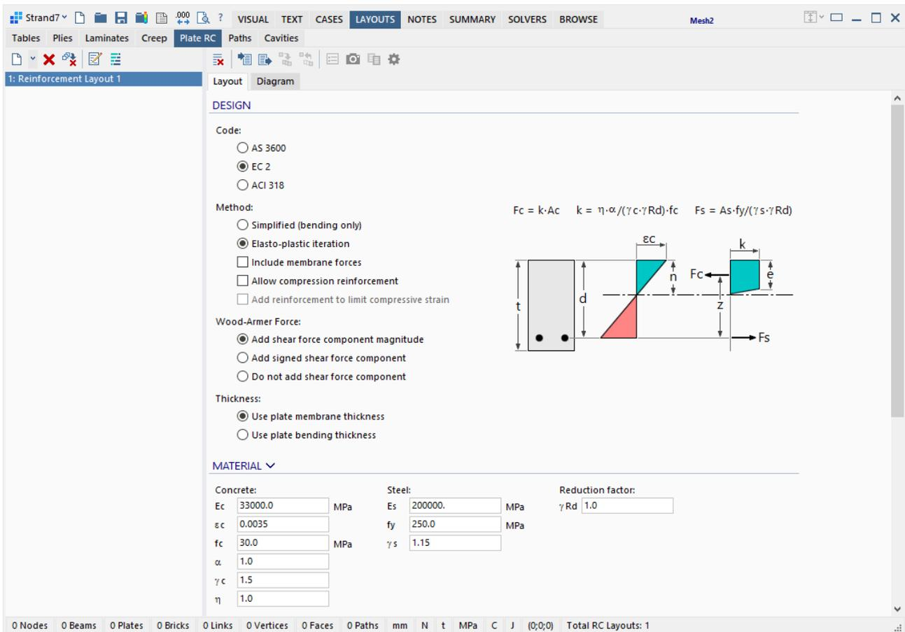
The **MATERIAL** section offers a popup menu with a range of standard steel and concrete properties, depending on the selected code.
