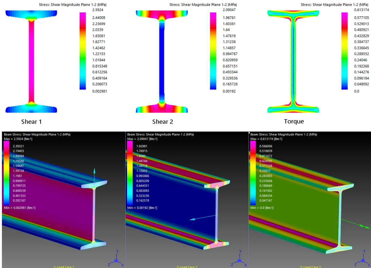
With the availability of shear stress on any cross section, R3 extends the previously available **Fibre Stress** yield criterion to include **Tresca** and **von Mises** criteria when a stress-strain table is assigned for material nonlinear analysis.
