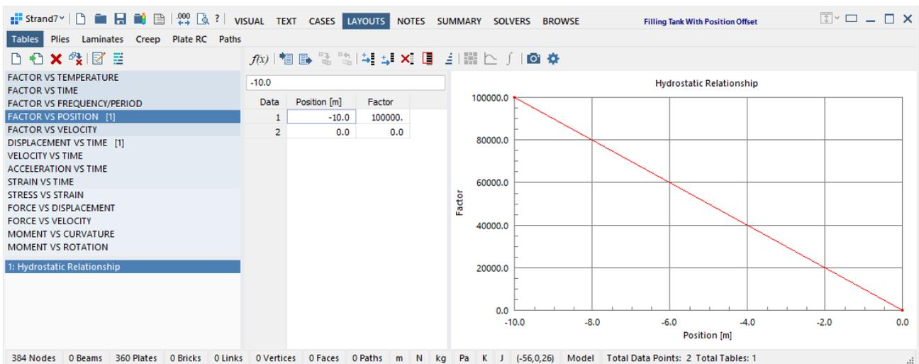
A Displacement vs Time table represents the relative movement of the tank with respect to the Factor vs Position table. This simulates filling over one second and then emptying.
