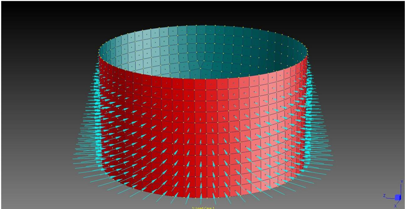
This feature is applicable not only to geometry, but also to elements. If applied to plate elements, a subdivision operation will re-evaluate all of the attributes on the new elements.
