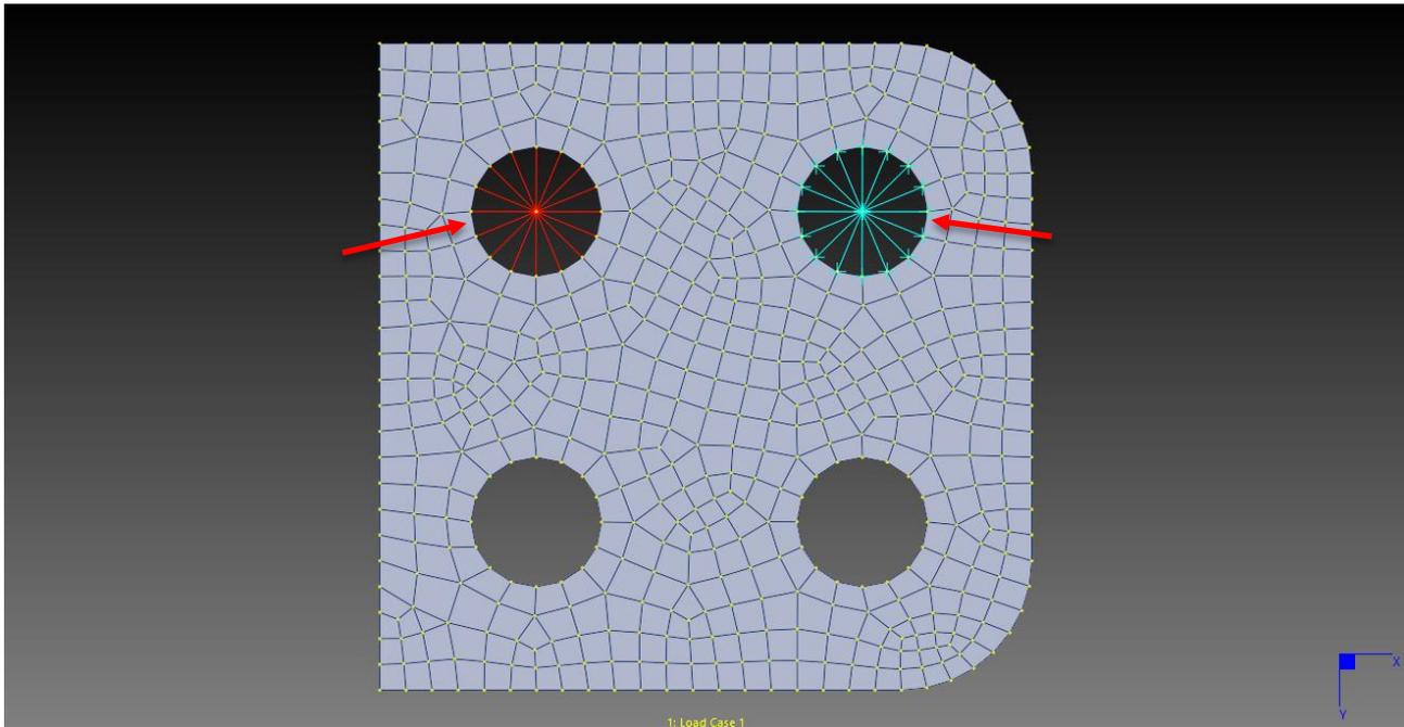
A tool is available to convert an MPL into the equivalent 2-node link cluster.
