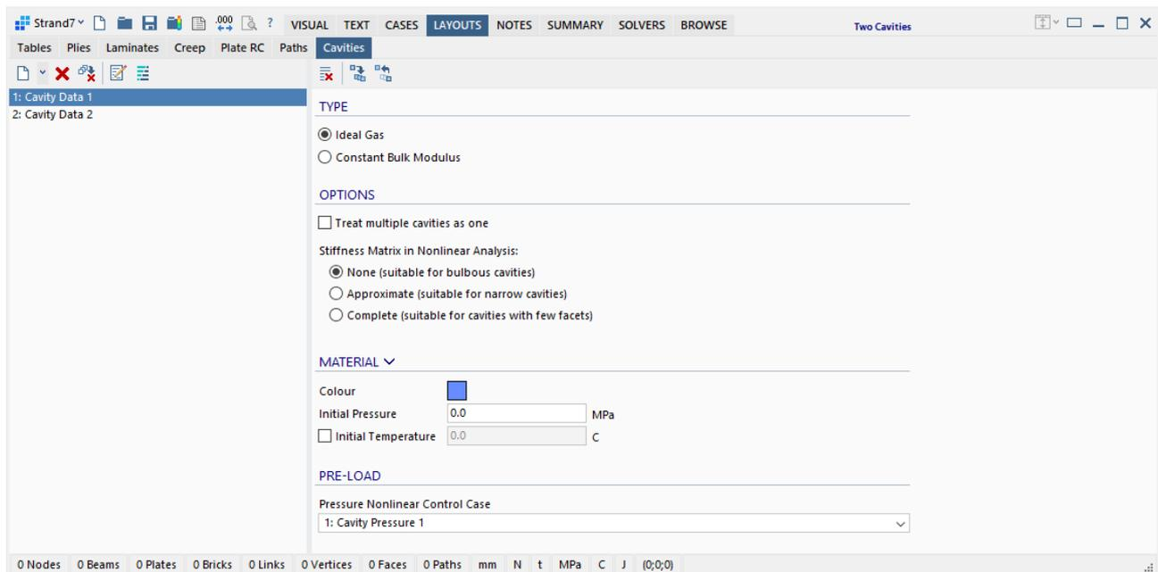
Two types of cavities are available and these are defined under **LAYOUTS/Cavities**:
