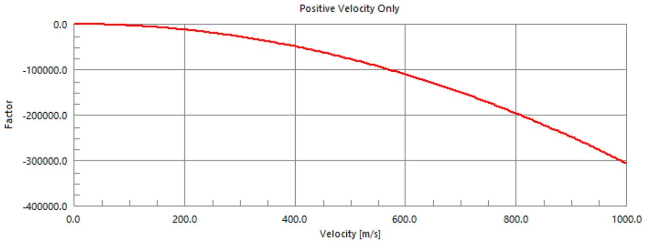
Alternatively, the table for both positive and negative relative velocity can be defined, and this will apply the drag pressure on both sides of the sphere in the travel direction: compressive pressure on the leading surface and suction pressure on the trailing surface. For this two-side approach, the drag equation magnitude needs to be factored by half because now the pressure is acting simultaneously on both sides of the sphere – this is shown below.
