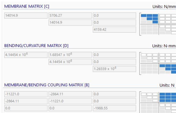
Without support for membrane-bending coupling, the [B] matrix is ignored and therefore a membrane force produces no out-of-plane bending, as illustrated below.
